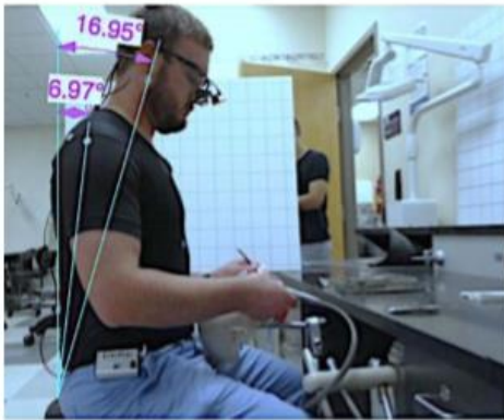
Figure 6: Posture Shirt –Side with angulation measurements.
